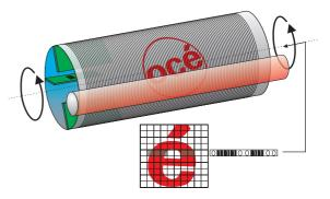
Figure 1. Direct conversion of digital data into toner-image. Schematically shown is a DI-drum with conductive tracks and a toner development roller.
